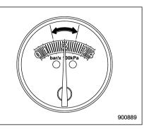
6. Turn the air compressor power switch off when the air pressure reaches the green zone of the air gauge.
