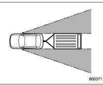
Many countries have regulations requiring special outside mirrors when towing a trailer. After hitching a trailer to your vehicle, check that the standard side mirrors provide a good rearward field of view without significant blind spots. If significant blind spots occur with the vehicle's standard side mirrors, use additional outside mirrors that conform with regulations.
