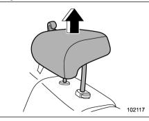
1. Raise the head restraint to the extended position. Do not remove the head restraint.
