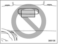
Do not attach labels or stickers to the windshield glass near the camera.
