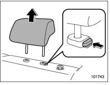
1. Adjust the head restraint as follows. (Except for center seat)
