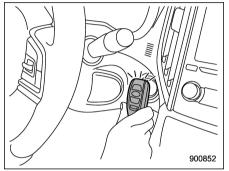
4. Hold the access key fob with the buttons facing you, and touch the push-button ignition switch with it.
