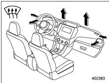
To turn on the defrost mode, press the defroster button " $\mathfrak{W}$ ", or select the " $\mathfrak{W}$ " position using the airflow mode selection button.
