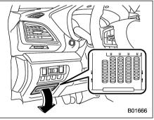
One is located under the instrument panel behind the fuse box cover on the driver's seat side. To remove the cover, pull it out.
