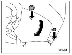
1. Remove the 2 clips and turn over the mud guard.
