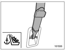
10. If the child restraint system requires a top tether, latch the hook onto the top tether anchorage and tighten the top tether. For additional instructions, refer to "Top tether anchorages" @ 1-44.
