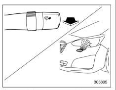
If you pull the wiper control lever toward you and hold it for more than 1 second with the ignition switch in the "ON" position, the headlight washer operates together with the windshield washer in the following conditions.
