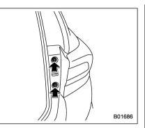
2. Using a Phillips screwdriver, remove the upper and lower screws that secure the rear combination light assembly.
