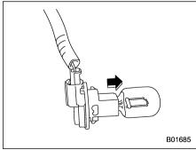
3. Pull the bulb out of the bulb socket and replace it with a new one.
