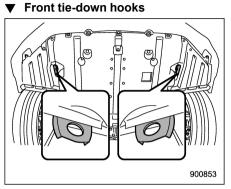
The front tie-down hooks are located between each of the front tires and the front bumper.
