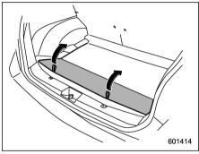
1. Raise and fold the rear end of the cargo floor board.
