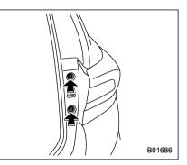
8. Tighten the upper and lower screws.
