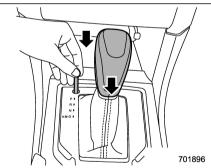
4. While depressing the brake pedal, insert a screwdriver into the hole, move it right and left while pushing the shift lock release button using a screwdriver, and
