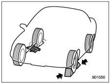
4. Put wheel blocks at the front and rear of the tire diagonally opposite the tire to be
