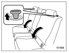
2. Unlock the seatback by pulling the lock release knob and then fold the seatback down.
