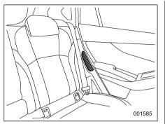
High voltage battery air intake
