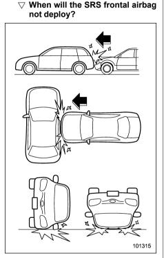
The SRS frontal airbag is not designed to deploy in most cases if the vehicle is struck from the side or from behind, or if it rolls onto its side or roof, or if it is involved in a
