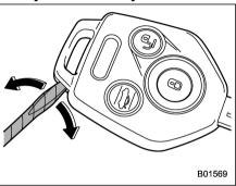
1. Wrap a flat-head screwdriver with vinyl tape or a cloth. Open the key head using the flat-head screwdriver.
