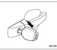
3. Insert the key into the key cylinder of the driver's door, then turn it in the locking direction to set the double locking system. All of the doors and the rear gate will be locked.
