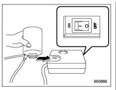
3. Turn the bottle upside down and tilt the bottle cap into the bottle holder of the air compressor.
