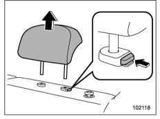
1. Adjust the head restraint as follows. (Except for center seat)
