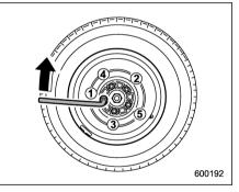
14. Use the wheel nut wrench to securely tighten the wheel nuts to the specified torque, following the tightening order in the illustration.
