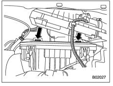
7. To install the air cleaner case (rear), insert the three projections on the air  $% \left( {\left[ {{{\rm{cl}}_{\rm{cl}}} \right]_{\rm{cl}}} \right)$
