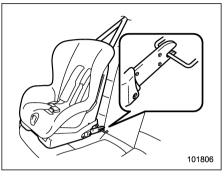
Your vehicle is equipped with ISOFIX anchor bars that allow an approved ISOFIX child restraint system to be installed on the rear seat without use of a seatbelt.
