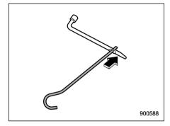
8. Insert the jack handle into the hole of the wheel nut wrench.
