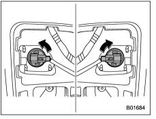
2. For left side light, turn the bulb socket clockwise and remove it.
