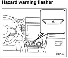
The hazard warning flasher is used to warn other drivers when you have to park your vehicle under emergency conditions. The hazard warning flasher works with the ignition switch in any position.
