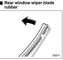
1. Pull out the end of the blade rubber assembly to unlock it from the plastic support.
