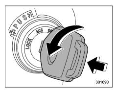
• To turn the key from the "ACC" to "LOCK" position, the select lever must be in the "P" position and the key must be pushed in and turned.
