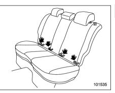
The ISOFIX anchor bars allow you to install a child restraint system only on the rear seat window-side seating positions. For each window-side seating position, two anchor bars are provided.
