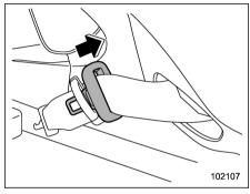
2. Remove the tongue plate from the belt holder and pull out the seatbelt slowly.
