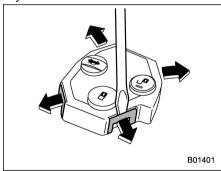
3. Open the transmitter case by releasing the hooks.
