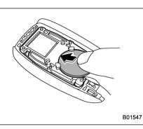
4. Insert a new battery with its positive (+) side facing upward as shown in the figure.
