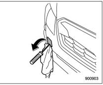
2. Cover the tip of a flat-head screwdriver with vinyl tape or cloth so that it will not scratch the bumper. Insert the flat-head screwdriver into the cutout of the cover and pry open the cover.
