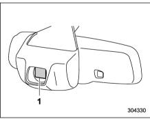
1) Camera for High Beam Assist function
