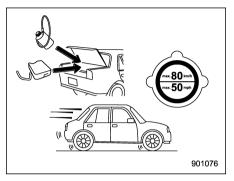
7. Stow the kit back in the vehicle and drive your vehicle immediately for 10 minutes or 5 km (3 miles).
