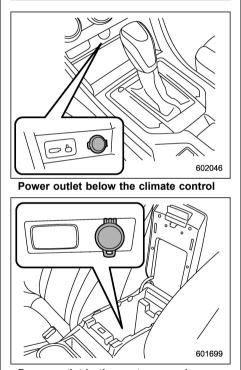
**Power outlet in the center console** Electrical power (12 V DC) from the 12 V auxiliary battery is available at any of the outlets when the ignition switch is in either the "ACC" or "ON" position.
