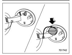
4. Set the fuel filler cap on the cap holder inside the fuel filler lid.
