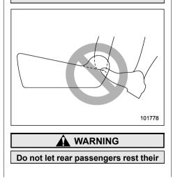
feet between the front seatback and seat cushion. Doing so may lead to defective operation of the following systems and could result in serious injury.
