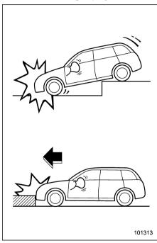
The SRS frontal airbag may be activated when the vehicle sustains a hard impact in the undercarriage area from the road surface (such as when the vehicle plunges into a deep ditch, is severely impacted or knocked hard against an obstacle on the road such as a curb).
