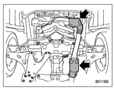
The catalytic converter is installed in the exhaust system. It serves as catalyst to reduce HC, CO and NOx in exhaust gases, thus providing cleaner exhaust.
