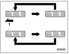
Models equipped with unidirectional tires 1) Front
