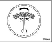
Turn the air compressor switch on and adjust the air pressure to the appropriate level (green zone of the air gauge).
