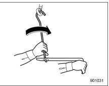
4. Tighten the towing hook securely using the jack handle and wheel nut wrench.
