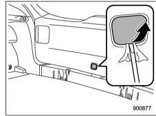
1. Remove the access cover at the bottom-center of the rear gate trim using a flat-head screwdriver wrapped with vinyl tape or cloth.
