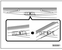
2. Turn the wiper blade assembly counterclockwise.
