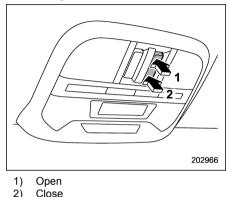
To open or close the sunroof using the automatic function, press and hold the switch toward the open/close side and release.
