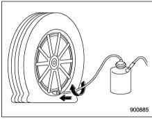
Connect the hose from the bottle to the tire valve stem tightly.
