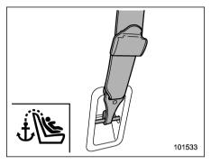
2. Attach the top tether hook to the appropriate upper anchorage.
