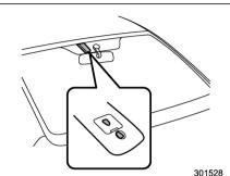
The sensor is on the windshield glass as shown in the illustration.
