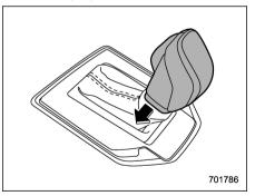
With the vehicle either moving or stationary, move the select lever from the "D"
