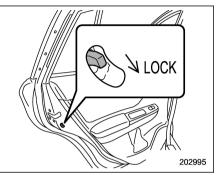
Each rear door has a child safety lock. When the child safety lock lever is in the "LOCK" position, the door cannot be opened from inside. The door can only be opened from the outside.
