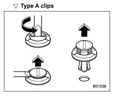
1. Turn the clips counterclockwise using a flat-head screwdriver until the center portion of the clip is raised.
