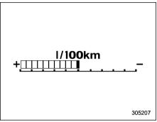
The ECO gauge shows the difference between the current rate of fuel consumption and the average rate of fuel consumption since the trip meter was last reset.
