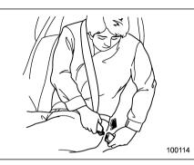
5. Insert the center seatbelt tongue plate in the center seatbelt buckle marked "CENTER" on the left-hand side until it clicks.
