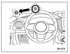
5. While filling the tire with air, attach the speed limit label on the position shown in the illustration.
