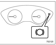
Auto Vehicle Hold operation indicator light While the vehicle is kept stopped by the Auto Vehicle Hold function, the Auto Vehicle Hold operation indicator light will illuminate.
