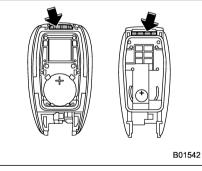
5. Attach the cover to the access key fob by fitting the projections and recesses together.
