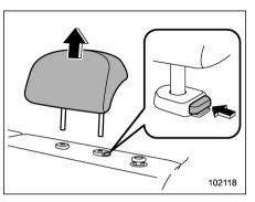
2. Remove the head restraint of the rear seating position where the child restraint system is to be installed.
