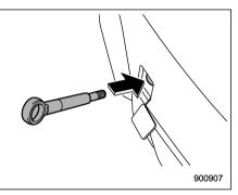
3. Screw the towing hook into the threaded hole until its thread can no longer be seen.
