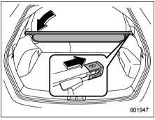
1. Insert the right end of the cover into the recessed portion with the arrow mark facing upward.
