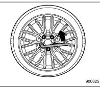
6. Loosen the wheel nuts using the wheel nut wrench but do not remove the nuts.
