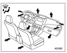
**Heat-def:** Windshield defroster outlets, foot outlets and both side outlets of the instrument panel (Refer to "Defrosting" #4-8.)
