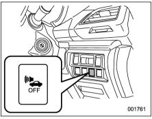
Pedestrian alert system OFF switch (RHD models)
