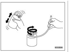
1. Shake the sealant bottle well. Loosen the hose.
