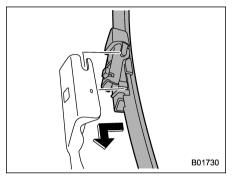
3. When installing the wiper blade assembly, align it with the wiper arm connection part and then slide it in the opposite direction of removal to install. After installing the wiper blade assembly, check that the connection part is locked completely.
