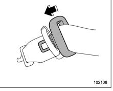
3. Allow the retractor to roll up the belt. You should hold the webbing end and guide it back into the retractor while it is rolling up. Then, pass the webbing under the belt holder and insert the tongue plate into the holder.
