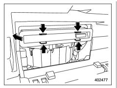
3. Replace the cabin air filter with a new one.
