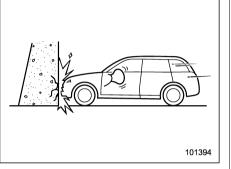
A head-on collision against a thick concrete wall at a vehicle speed of 20 to 30 km/h (12 to 19 mph) or higher activates the SRS frontal airbag. The SRS frontal airbag will also be activated when the vehicle is exposed to a frontal impact similar in fashion and magnitude to the collision described above.
