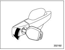
Insert the key into the key cylinder of the driver's door, then turn it in the unlocking direction to cancel the double locking system. All of the doors and the rear gate will be unlocked.
