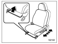
Pull the lever upward and slide the seat to the desired position. Then release the
