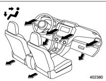
**Bi-level:** Instrument panel outlets and foot outlets
