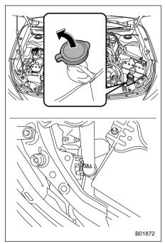
Remove the washer tank filler cap, then add windshield washer fluid until it reaches the "FULL" mark on the tank.
