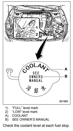
1. Check the coolant level on the outside of the reservoir while the engine is cool.
