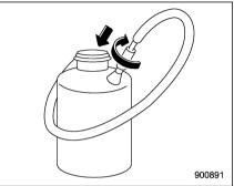
Connect the hose of the bottle to the valve of the bottle in a circular fashion to avoid leakage of the remaining sealant.
