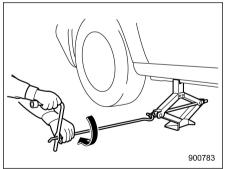
9. Insert the jack handle into the jackscrew, and turn the handle until the tire clears the ground. Do not raise the vehicle higher than necessary. 10. Remove the wheel nuts and the tire to be replaced.
