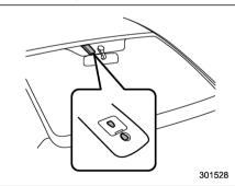
The rain light sensor is on the windshield glass.
